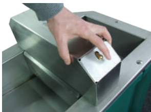
Valve cover can be opened without use of tools
