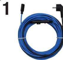
Check the heating cable before installation (isolation and resistance). The thermostat must be cooled with ice cubes or ice spray to measure. Note the results in the table, and check the resistance according the table at "technical data".
